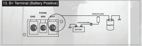
Due to the power requirements of the amplifier, this connection should be made directly to the positive (+) terminal of the battery. For safety purposes, install an in-line fuse holder (not included) as close to the battery positive (+) terminal as possible with an ampere rating not to exceed the total value of fuses in the amplifier.
